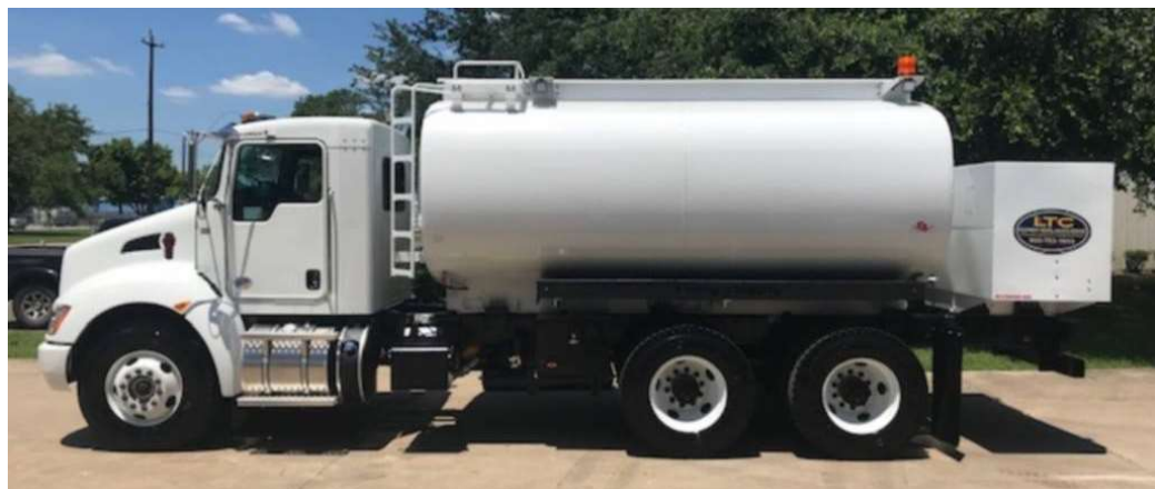
b) Mobile fueling drops for on-site equipment
